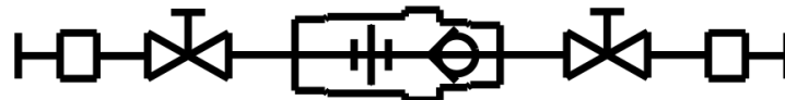
Circuit Solver Union Assembly with Pro Press Ends (CSUA-PP) and integrated Check Valve 1)
