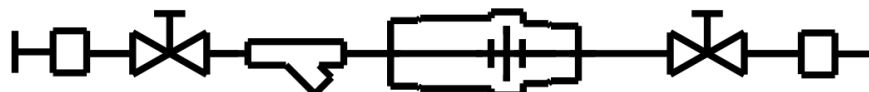
Circuit Solver Union Assembly with Pro Press Ends (CSUAS-PP) with integrated Strainer 4)
