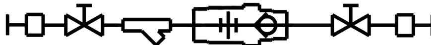
Circuit Solver Union Assembly with Pro Press Ends (CSUAS-PP) with integrated Check Valve 1) and Strainer 4)
