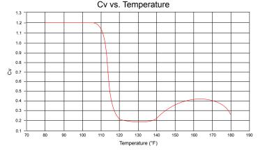
This dual balancing thermal disinfection valve is typically used when the entire domestic hot water system is being thermally disinfected at once. This provides the opportunity to limit the amount of flow of the 160°F disinfection temperature water as it approaches 170°F in each branch/riser.
