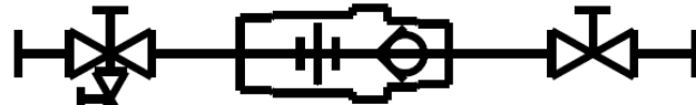
Circuit Solver Union Assembly (CSUA-W) with integrated Check Valve 1) and side drain inlet ball valve 5)
